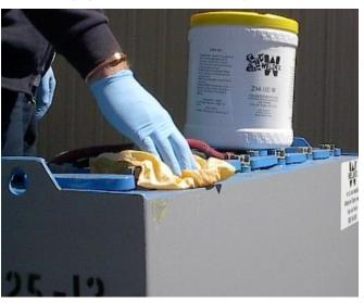
One of the main causes for battery damage is corrosion caused from electrolyte on the surface of the battery. If the electrolyte (acid) stays on the surface it causes electrical shorts, and causes white battery corrosion between the cells. Acid & corrosion on the surface is hazardous to the operator. The build up of corrosion between the cells grows until it puts pressure on the cell walls and eventually destroys it. The corrosion will eventually damage the lift.
