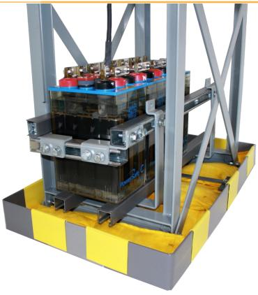
**Angles, corners, and over clips:** ½ inch thick gray PVC plastic and 4 inches tall as required in the National Fire Code. All PVC components have a LOI flame rating of 28 or higher which meets the requirements of UL standard 2436.
